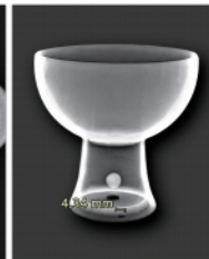
Defected Porcelain (Hole)
