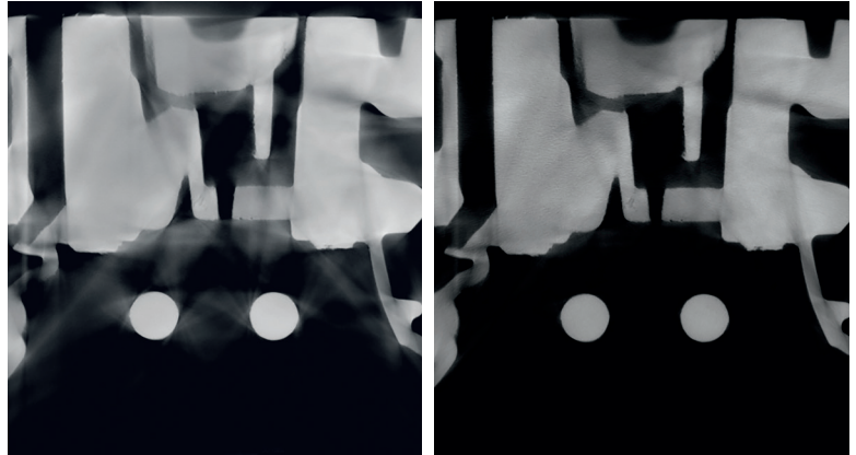
Improving image quality: Cone-beam CT without (left) and with ScatterFix 2.0 (right).
