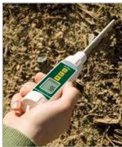
Includes 8" (20 cm) stainless steel moisture probe
