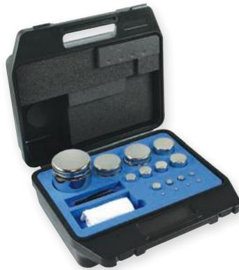
Test weight material: Polished stainless steel
