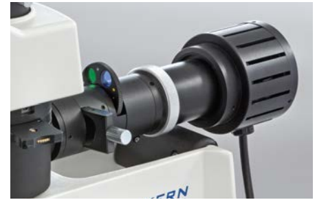
Illumination unit with filter disc
