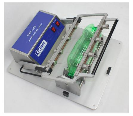
The "CanNeed-HWC-100 Hot Wire Bottle Cutter" offers an easy-to-use and cost-effective method for cutting containers for section weight analysis. It can cut PET bottle into several determined sections (The maximum is up to 5 sections). Then, the user can check whether each section accord with the corresponding weight standard. CanNeed-HWC-100 can quickly cut PET bottle with hot wires. Clear profiles can be obtained without PET deformation. PET bottle samples can be 200-3000 ml.
