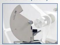
Existing model 83-11 Elmendorf Tear Tester pendulums are compatible with the new 83-76 unit, preventing the need for additional pendulums.
