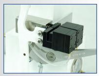
Simple, two-button operation of the pneumatic clamp and swing ensures efficient testing. A built-in cutting blade prepares samples quickly and easily.
