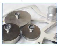
A universal pendulum with quick change hardware and weights provides multiple testing options. The required calibration weights are also included.
