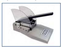
The **83-20-08 Sample Cutter** produces rectangular samples for paper and textile testing based on ASTM D 689 and TAPPI T 414 specifications.
