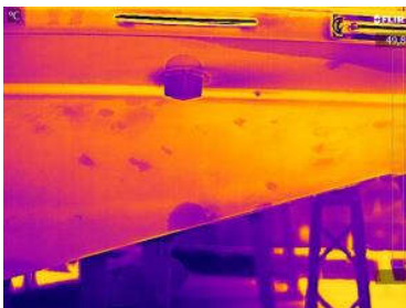
Thermographic analysis on boat keel - Halogen lamps
