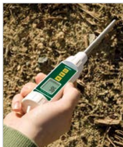
Includes 8" (20 cm) stainless steel moisture probe
