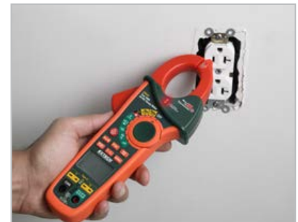
Non-Contact Voltage (NCV) Detection.
