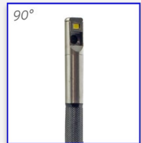
90° direction fixed objective available up to 10 meter length. Ideal For NDT welding Inspections
