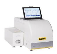
and control the temperature, humidity and flow rate precisely, which guarantee the testing sensitivity and repeatability of test results. C390H is applicable to determination of water vapor permeability of plastic films, sheeting, paper, packages and other relative packaging materials in food, pharmaceutical, medical apparatus, consumer goods, photovoltaic and electronic industries, etc.
