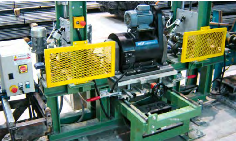
Steel bar inspection with EC100 rotor
