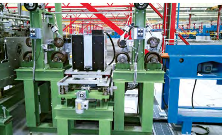
Inspecting wires / bars using encircling coils
