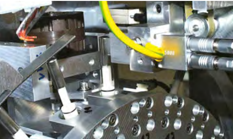
Crack inspection on deep-drawn bushings
