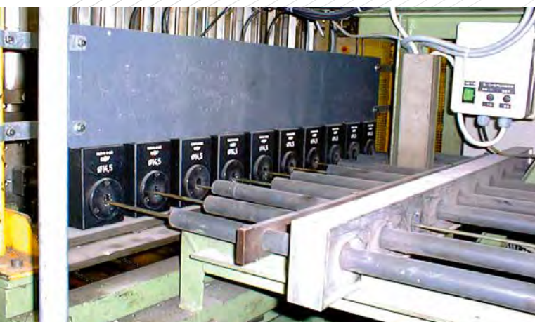
Multi-channel inspection with coils
