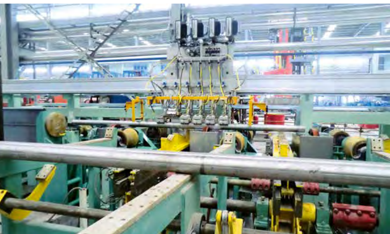
Eddy current and ultrasonic tube testing system
