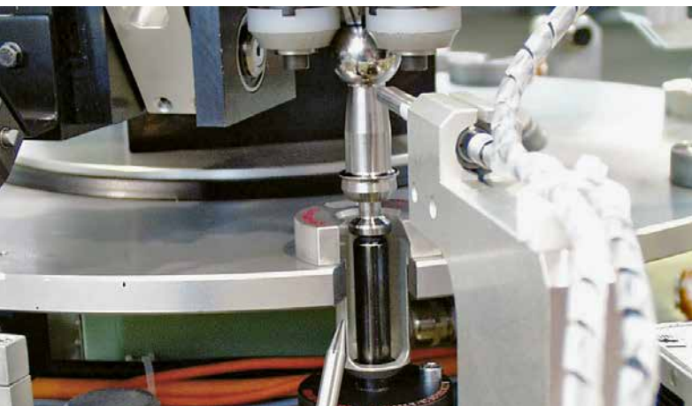
Fully-automatic crack detection on ball studs
