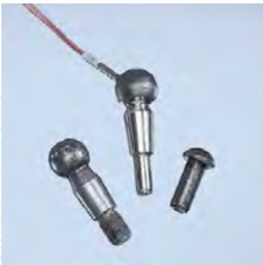
Manipulator-compatible miniature probes
