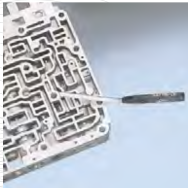
Crack detection on complex structures
