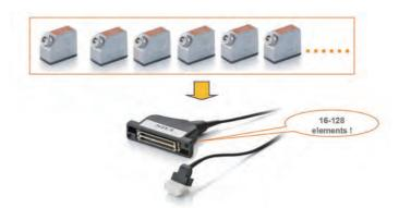
One phased array probe consists of many small elements, each one can be pulsed on separately. The structure of the phased array probe is like putting many single element probes into one probe.
