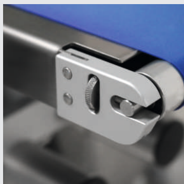
BELT ADJUSTMENT MECHANISM "WITH MEMORY" FOR EASY BELT REPLACEMENT
