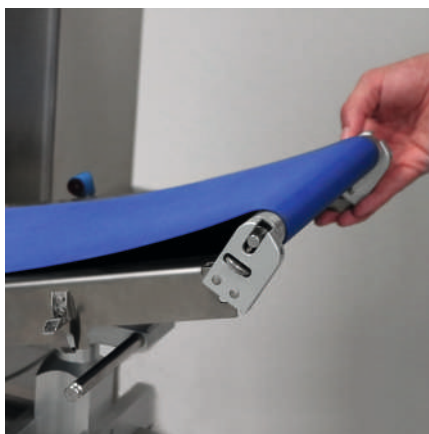
QUICK BELT DISASSEMBLY SYSTEM
