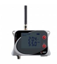
GSM data logger is designed to record temperature and humidity from external probe. In case of exceeded set limits, SMS and JSON messages can be sent via GPRS data connection. It is possible to set the regular sending of JSON messages to COMET Database, the sending interval is adjustable. Alarms are also indicated locally by LED, LCD and acoustically by built-in beeper.
