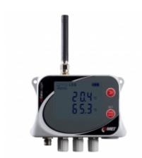
GSM Datalogger is designed to record temperature from four external Pt1000 probes. In case of exceeded set limits, SMS and JSON messages can be sent via GPRS data connection. It is possible to set the regular sending of JSON messages to COMET Database, the sending interval is adjustable. Alarms are also indicated locally by LED, LCD and acoustically by built-in beeper.
