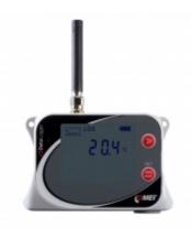
GSM datalogger is designed for temperature recording. In case of exceeded set limits, SMS and JSON messages can be sent via GPRS data connection. It is possible to set the regular sending of JSON messages to COMET Database, the sending interval is adjustable. Alarms are also indicated locally by LED, LCD and acoustically by built-in beeper. The recording is performed in a non-volatile electronic memory. The data can be transferred to a PC via USB-C.
