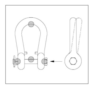
The shackles should be examined regularly by a qualified person. The time interval from one check to another depends on how much the instrument is used, but it is recommended to not exceed six months.
