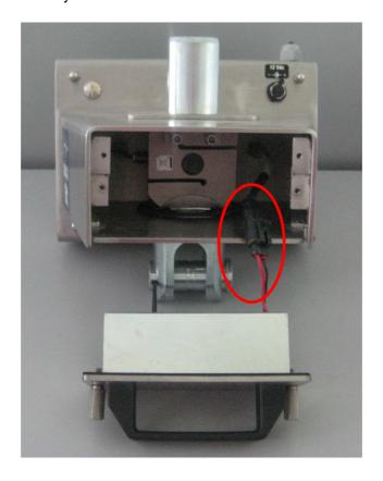
4) Unplug the connector automotive AMP from the battery pack.
