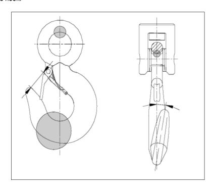
The eye hook should be examined periodically by a competent person. The interval among the inspections depends on the frequency of use of the instrument, but it is recommended not to exceed six months.
