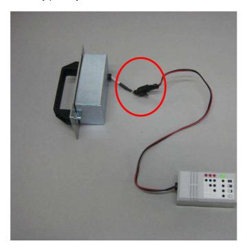
6) Insert the power supply (12Vdc) to the network at 230Vac and plug the charger by the connection jack.
