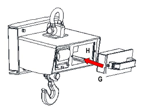
**G:** Are the battery box and the relative way of insertion in the electronic crane scale MCW. **H:** is the insertion slot in which you insert the battery box. The slot is located on the back of the instrument.
