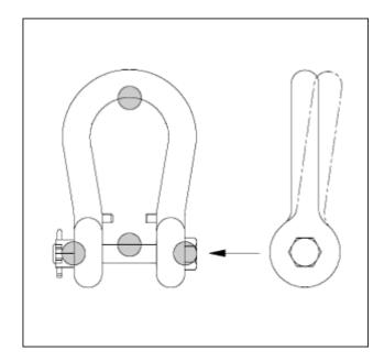
The shackles should be examined regularly by a qualified person. The time interval from one check to another depends on how much the instrument is used, but it is recommended to not exceed six months. Therefore, one must:
