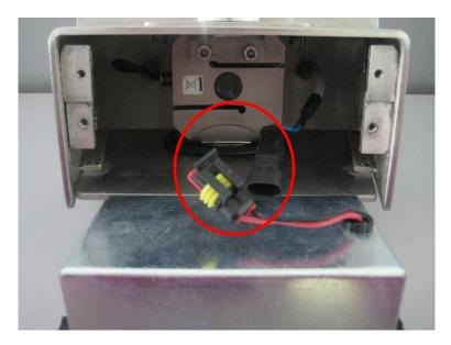
5) Connect the charger to the battery pack by the auto-motive AMP connector.
