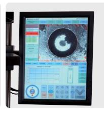
NEXUS 3001XLM-IMP can also be operated as a Brinell indentation press only. Without the use of the IMPRESSIONS<sup>TM</sup> interface. NEXUS 3001XLM-IMP is standard equipped with an automatic motorized spindle for a fully automatic testing procedure. IMPRESSIONS™ video indent measurement system and tester user interface offers unlimited testing results storage capacity and allows to set up a number of standard test programs.
