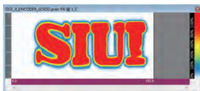
C Scan In-Amplitude, showing echo amplitude
