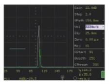
Refresh the highest echo within the screen range automatically, completing flaw positioning quickly.
