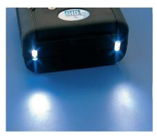
atmosphere prior to entry, the flashlight can be used to illuminate the water surface, avoiding immersing the instrument in potentially damaging or dangerous chemicals or sewage. The existing battery unit of the G450 can be replaced with an integrated lamp battery unit if necessary. Thus, an easy upgrade is guaranteed.
