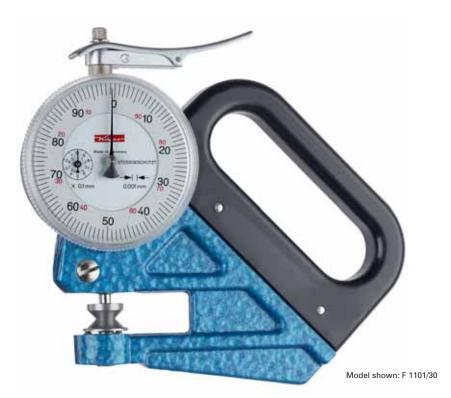
These handy instruments are used exclusively to measure the thickness of thin foils. The frame has the required rigidity, the insulation of the handle prevents transfer of heat from the hand of the user to the sensitive mechanical parts of the Dial Gauge.
