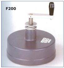
The accuracy of test results is not only dependent on the accuracy with which the procedure is carried out, but also on the accuracy of cutting the test pieces (specimens) from the original sample. Some tests, for example, tensile strength and edge crush, are particularly sensitive, and cutting accuracy is a prime cause of variation in the values obtained. These precision cutters are designed to eliminate the causes of errors associated with hand-cut samples.
