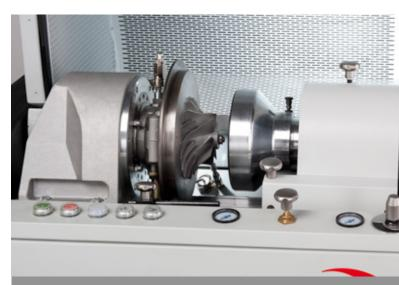
The wide weight range extends your business The TB sonio and the TB comfort are matched with each other so that turbocharger components and core assemblies up to 16 kg can be perfectly balanced. Just two machines can now balance turbochargers for commercial vehicles, construction machinery and marine engines.
