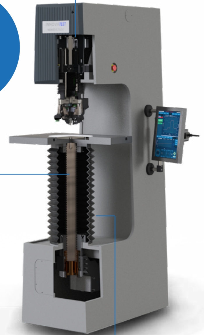
Z-AXIS BALL SCREW Precision movement
