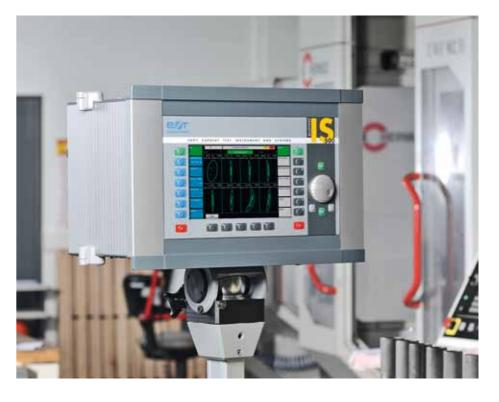
The main feature of the new family of instruments is the fully digital signal processing chain with an extremely wide bandwidth starting from 10 kHz and with an ultra-fast multiplexing rate of a 32 kHz (probe to probe).
