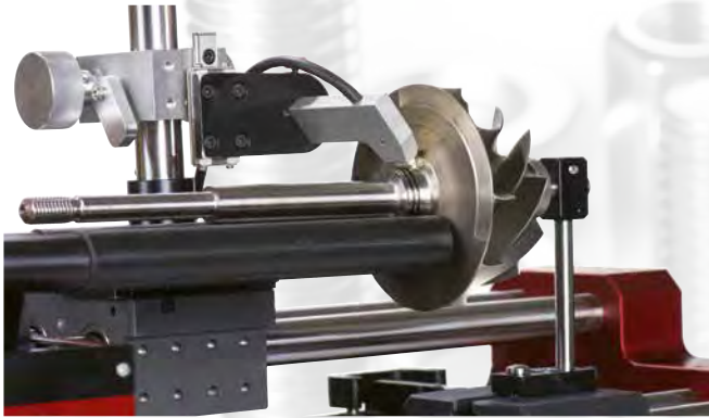
Crack testing with inclined test probe in the bearing seat area
