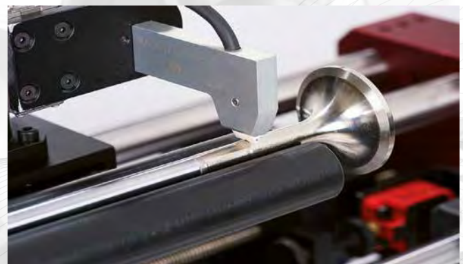
Crack test cylinder surface and friction weld sea
