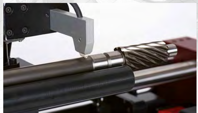
Crack testing in the puncture area
