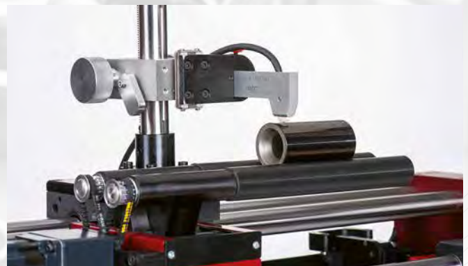
Crack testing on a ground surface
